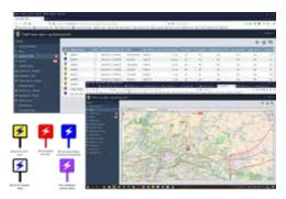
Picture on the left: View of the dispatcher screen showing the switching points in the form of a table or a map. Different colours of the icons determine the basic states of the relevant switching point.
