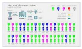
The superior level of the charging infrastructure equipped with Foxtrot is a web application with a user interface, which provides an overall overview of the current charging state, provides historical data and statistics on the use of individual charging stations and it also manages individual users. The system allows the operator to change the limits as needed and based on the fact how the agreed reserved power input in the building changes and progresses.
